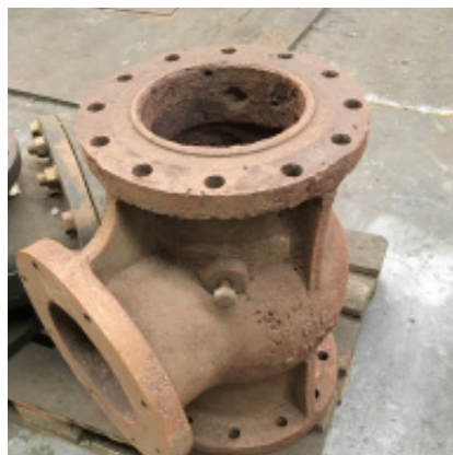
Picture 4: Original cast steel body after shot blasting
